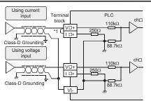
\*1 Make sure to short-circuit the 'V\(\pi\)+' and 'I\(\pi\)+' terminals when current is input.
